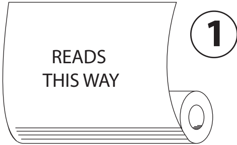
DIRECTION #1 Label on OUTSIDE of roll. Copy printed ACROSS the roll. Top of label OFF FIRST
